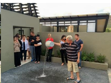
Demonstration of porous Hydromedia concrete driveway for water harvesting
